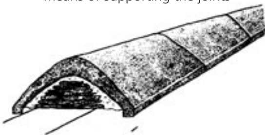
Stone ridge tiles showing the method of support
