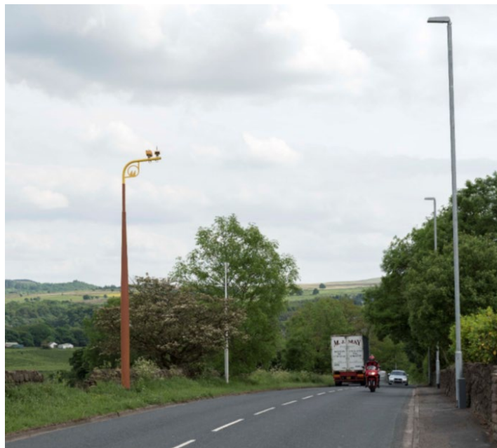
Photograph showing an alternative brown colour with yellow camera support arm, as an option. Overall, the conspicuity is reduced but there is still a visible presence.
